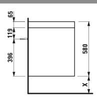
X =The exact height must be set during installation.
