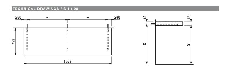
X = The exact hight must be set during installation.
