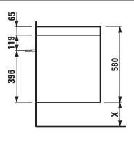
X = The exact height must be set during installation.
