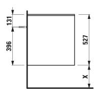
X = The exact height must be set during installation.
